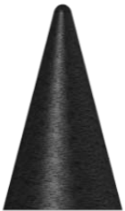
Initial Deformation Temperature (IT) Temperature at which the first rounding of the Apex of the cone occurs
